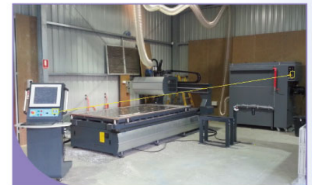
Me1050 Controller To LS-750E Remote Start-Stop Requirement
