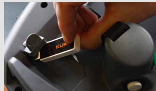
A USB port integrated into the housing allows the simple saving and loading of configurations directly on the smartPAD.
