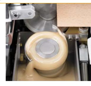
The KUPER glue application system featuring the almost horizontally installed glue application disc guarantees a precise glue application avoiding glue spots on the joint up to 100 %. Using this glue application system veneers in thicknesses of approx. 0.3 – 1.5 mm can be spliced.
