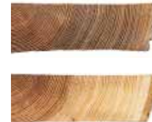
Smooth colour by thermal treatment e.g. if ash and beech wood with dark centre (heart) are treated.
