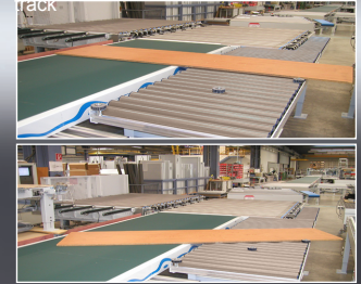
Return-conveying of long parts with automatic turning
