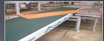
Return-conveying of long parts with automatic turning
