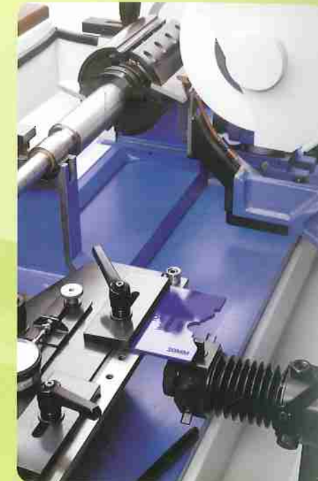
Multiple tracing rods allow for accurate and convenient grinding.
