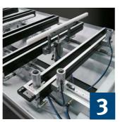
Machine table 10 supporting bars with mechanical clips
