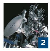
Tool changer Chain-type tool changing magazine with 12, 16, 24, 32 tool places
