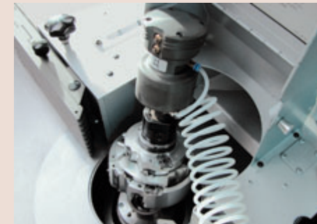
Quick cutter change system T 2660
