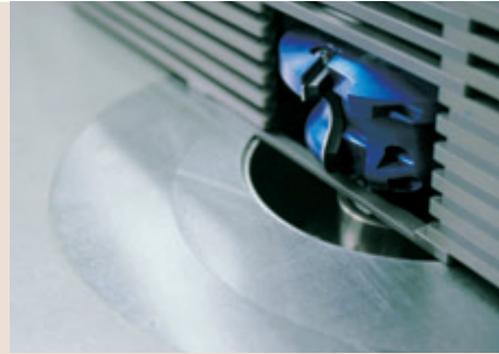
Electrically adjustable table opening
