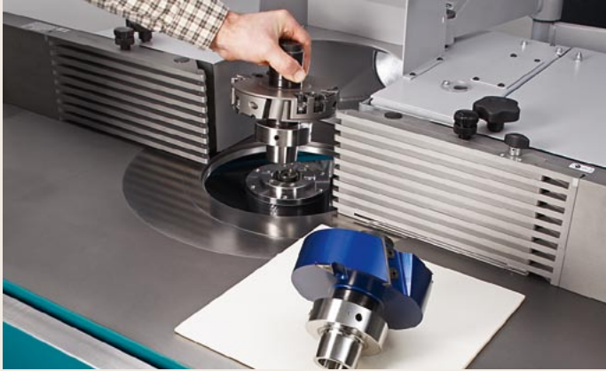
HSK cutter arbor quick change system
