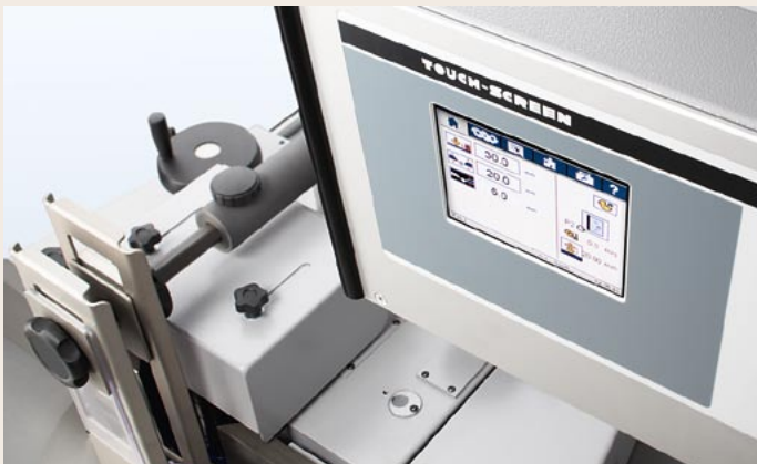
Digital display for the infeed fence jaw
