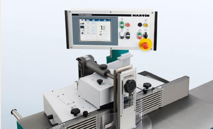
Electronic fence positioning
