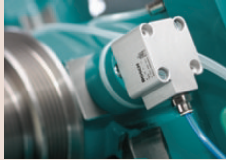
Electro-pneumatic saw arbor locking
