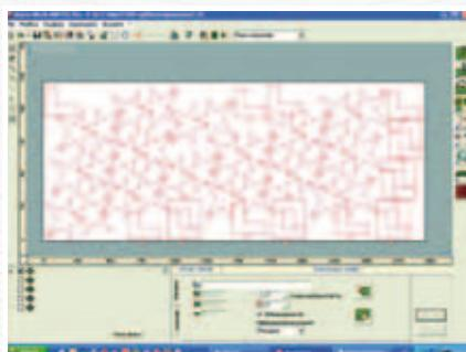
Software package for the automatic optimisation of the positioning of components to be machined on a single panel.
