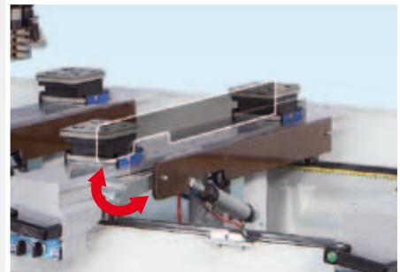
Panel lifting blades for easy positioning of heavy workpieces.
