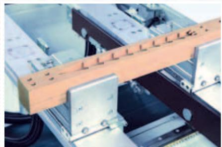
Mechanical clamping systems for solid wood, linear and arched components machining.
