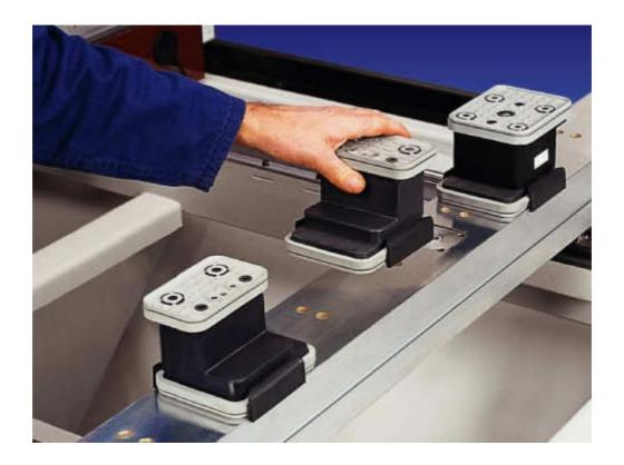
Suction cups positioning The vacuum-operated locking system of the cups dramatically reduces the working table setting time.
