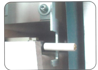
• Security switch by ceramic bars 砂帶安全開關
