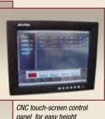
panel for easy height adjustment of one or multiple heads
