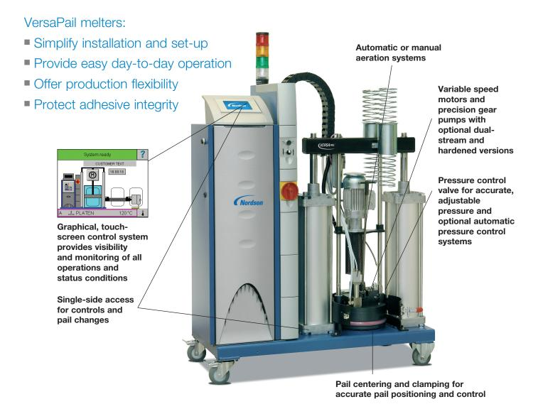
Nordson® VersaPail bulk melters are designed for precise demanding hot melt adhesive application from 20-liter or 5-gallon pails. With a variety of pump types and sizes, VersaPail melters are customizable to accommodate a wide variety of adhesives and meet specific manufacturing requirements. A powerful industrial PC provides full control of the adhesive system via a touch-screen interface and displays messages and indicators for each operator activity and every machine status condition.
