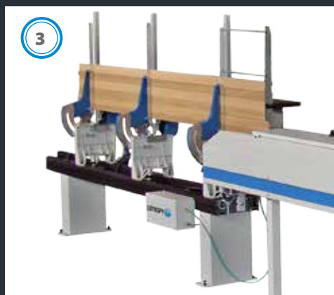
Pneumatic transfer conveyor belt 2000 x 600 mm
