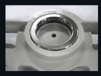
Ball bearing on swinging of saw arm for smooth and steady cutting action.
