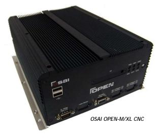
OPEN-M and OPEN-XL, respectively equipped with Intel Celeron-M 2.0 GHz CPU and Core 2 Duo 2.26 GHz, are suitable for the development of complex applications, having a computing power fitting the multi-process working centers with several axes. For both models, the SW structure with dual operating system Windows CE and Windows 7 (WES7) is available for the simultaneous execution, on the same hardware, of both CNC real time applications and market software for Windows<sup>™</sup>.
