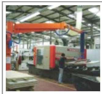
Knuckle Jib support gantry is suited to applications where there are restrictions to move around
