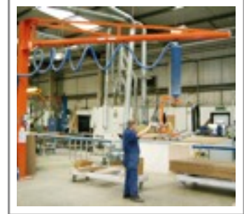
Lifting sheets from stack and rotating through 90 degrees to load a Vertical Panel Saw. 180 degree rotation is also available for inspection with manual and pneumatic options
