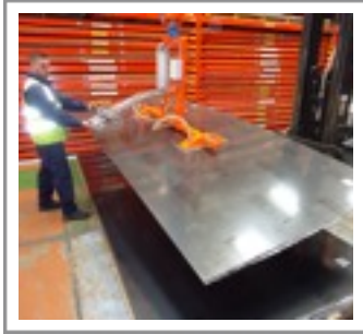
Lifting sheets from stack and rotating through 90 degrees to load a Vertical Panel Saw. 180 degree rotation is also available for inspection with manual and pneumatic options
