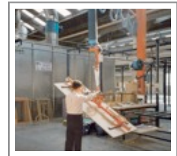
Lifting and turning doors using narrow suction pads
