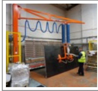
Lifting sheets from stack and rotating through 90 degrees to load a Vertical Panel Saw. 180 degree rotation is also available for inspection with manual and pneumatic options
