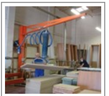
Swing Jib support gantry available from 2-5m
