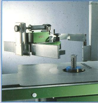
UK Device for pivoting the shaper fence aside through electric lifting up and down of the shaper fence.
