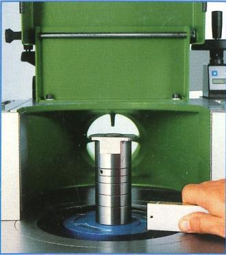
UK Zeromaster device for setting the reference measure for adjusting the zero-point on a new tool.
