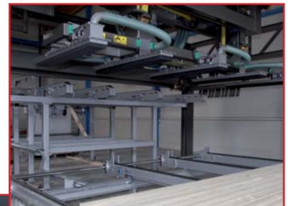
Fig. 14: Automatic destacking system
