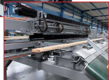
Fig. 16: Distribution to two cross-cut stations
