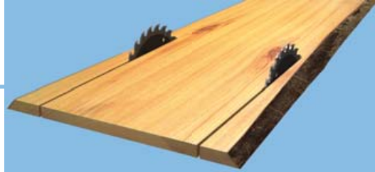
Fig. 7 Board edging in the edger
