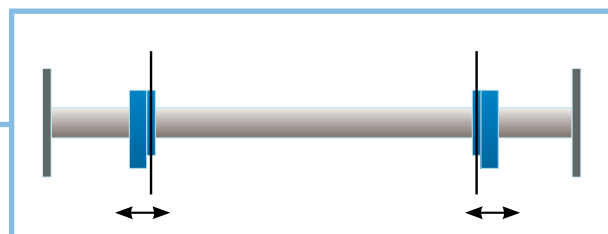
Fig. 2 Saw shaft with two moving saw bushes
