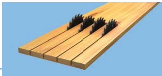
Fig. 9 Ripping of square-edged boards in the rip saw
