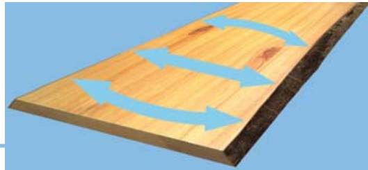
Fig. 6 Alignment of waney-edged boards in the automatic infeed system
