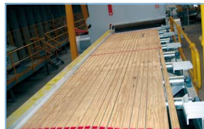
Fig. 4 Ripped LVL panels
