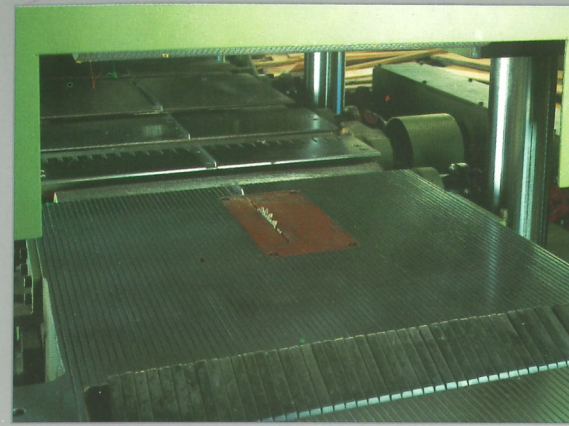
Scoring and guide system for straight line ripping, mounted on PMA2-MS machine
