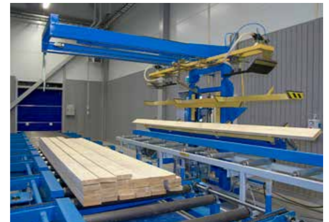
Timber picker with additional roller conveyor system
