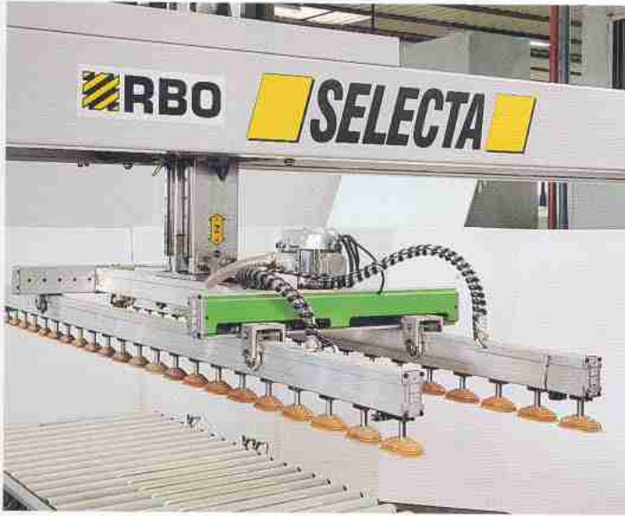
Numerically controlled regulation of the vacuum cup frame Digitale Rahmenverstellung
