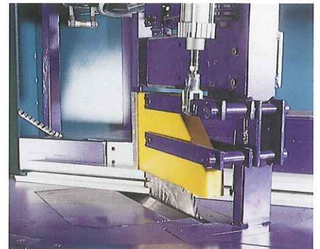
The system fitted with a special saw for angle cutting
