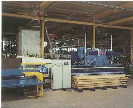
Automatic loading of the saw using a vacuum lift
