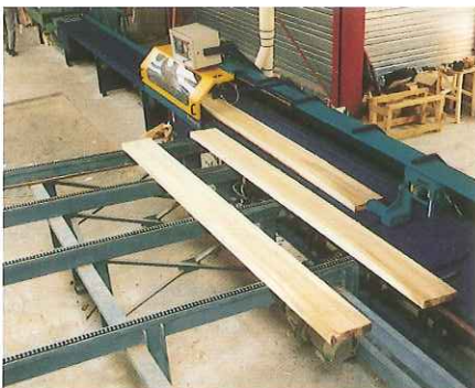
Fully automatic infeed loading conveyor used on a machine in the packaging industry.
