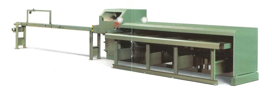
The workpiece is placed on the transverse conveyor and measured automatically by a scanner. At the same time the transverse conveyor acts as a buffer, from which the machine automatically collects the workpiece to be machined.
