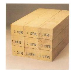
If required, the VARIO-LINE can be equipped with an ink-jet printer, which marks the cut workpieces (eg length and identification number or information specific to the firm).
