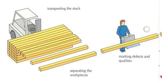
This schematic drawing shows the general construction of a REINHARDT VARIO-LINE optimization cross-cutting plant for trimmed workpieces.
