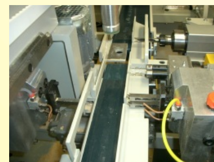
In the processing unit all the pieces are clamped. The width is positioned automatically
