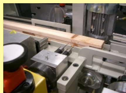
Inlet with buffer conveyor. The pieces are often coming directly from a moulder or a double ending tenor.
