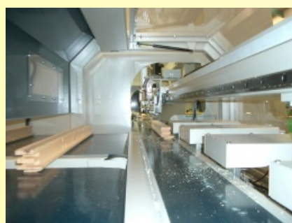
After processing the pieces they leave the unit on a outlet buffer conveyor belt.
