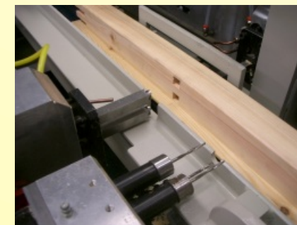
Two powerful servo motors will move the components at a high speed rate. Some of the processing units are fixed and others can move and reposition.
