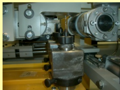
The components are moved one by one from the buffer conveyor onto the conveyor running into the processing unit.
