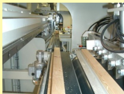
The components are moved one by one from the buffer conveyor onto the conveyor running into the processing unit.
