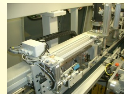
Two powerful servo motors will move the components at a high speed rate. Some of the processing units are fixed and others can move and reposition.
