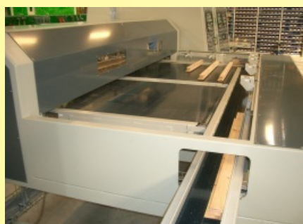
Inlet with buffer conveyor. The pieces are often coming directly from a moulder or a double ending tenor.
