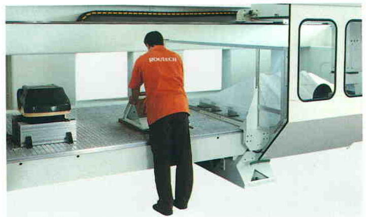
Central polycarbonate safety shield for pendulum machining.
