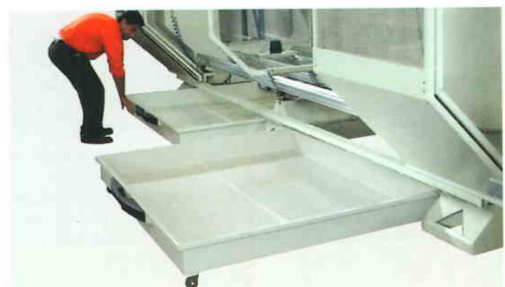
Central polycarbonate safety shield for pendulum machining.
