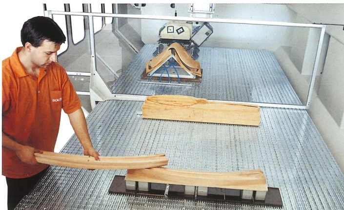
Central polycarbonate safety shield for pendulum machining.
