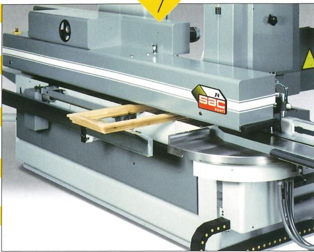
7) Sash profiled on external on profiling unit only
