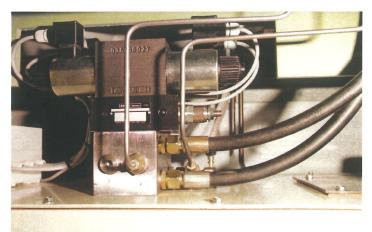
All **SAVI** guillotines are equipped with a central hydraulic block system, that minimizes the risk of leakages.
