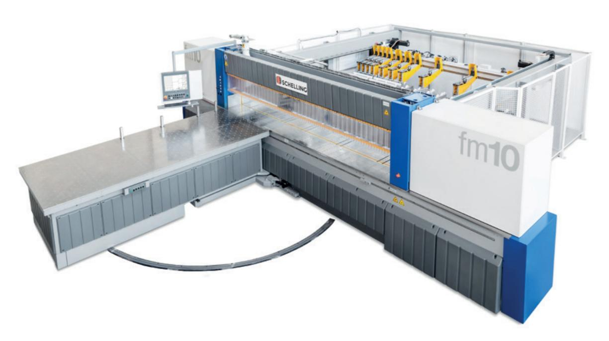
The patented turntable with 90° rotation makes saw operation even simpler and cutting more productive. Thirty years ago, Schelling invented the turntable and has continued to develop it ever since. Today, the entire machine is adapted to the turntable. It is mobile and semi-automatic. Quickly, plates and strips are first cut lengthwise, then crosswise.
