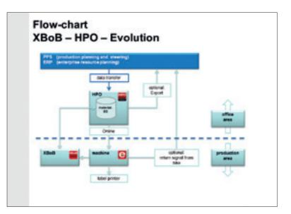
The operating data reporting of the MCS Evolution logs all relevant operating data, such as operating hours and the travel paths of the saw unit, feeder, pressure beam, etc. In addition, the running data of the saw blades are individually captured.
