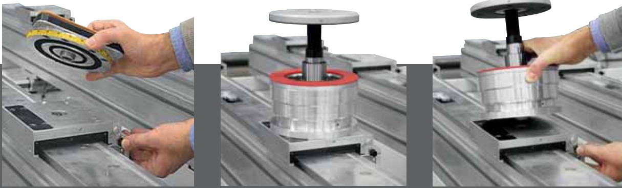
Switching from clamps to suction cups and vice versa is quick and easy. The quick coupling developed by SCM allows operators to change the accessory at the press of a button.
