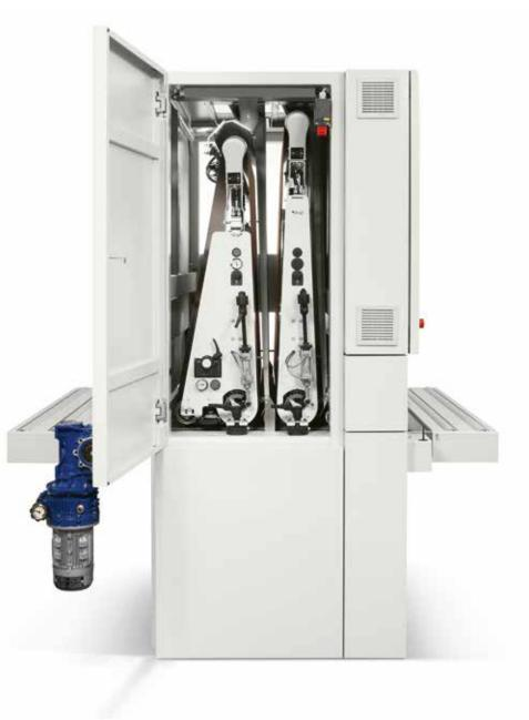
Belt oscillation controlled by an electronic photocell This precision control system guarantees maximum uniformity in belt oscillation: this reduces the risk of belt breakage and improves finishing quality.
