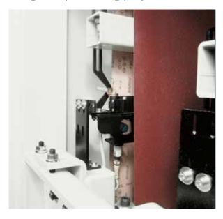
Automatic feed belt tensioning and centering: for an easy operation An electro-pneumatic system keeps the feed belt on track, perfectly centred and tensioned at all times. The system is automatic and no operator intervention is required.
