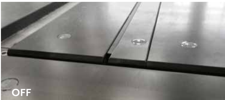
Automatic closure of the cutting line: it avoids the fall of waste trim cuts inside the machine.
