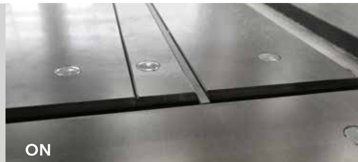
Automatic closure of the cutting line: it avoids the fall of waste trim cuts inside the machine.
