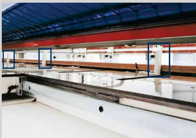
Front alignment devices for the automatic loading.
