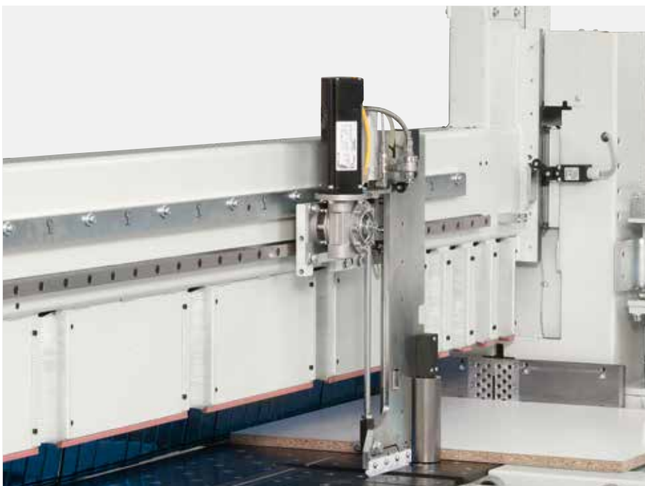
Powered side alignment device: drastic cycle time reduction and better grip of the piece by means of the brushless motor.
