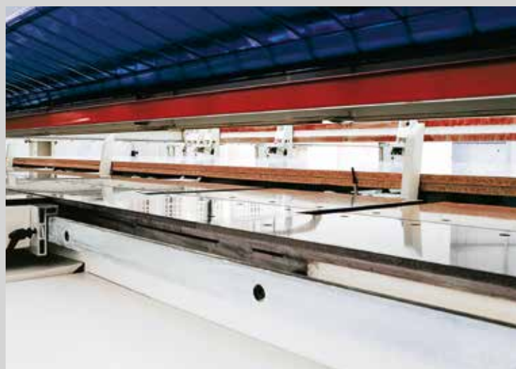
Front alignment devices for the automatic loading.
