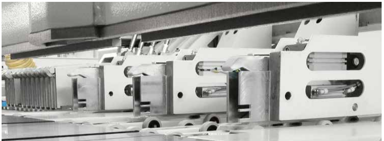
Clamps with on/off pneumatic stops for covered panels with overhanging edges.
