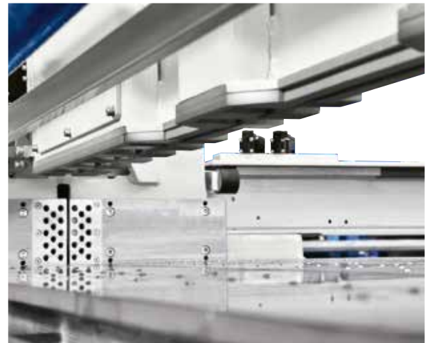
Front alignment devices for the automatic loading.
