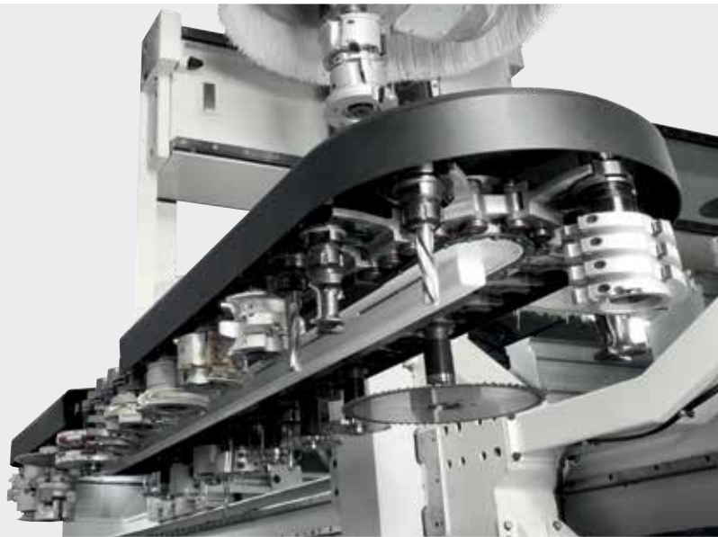
The machine can be fitted with toolholder-stores of up to 48 stations for each machining unit.
