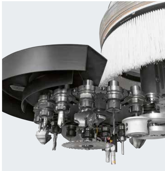
Many tools always available thanks to the R16 rear tool changer.
