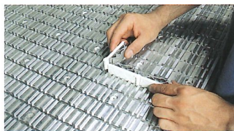
Easy worktable tooling. With three types of MPS suction cup, the practical MODULSET modular hold-down system and extra, electro pneumatically controlled perimeter stops
