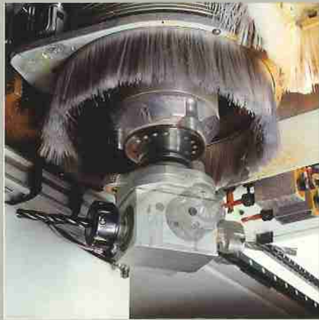
Vector rotary axis enables the use of special angle drive units which can achieve 0-360° rotation from the CNC
