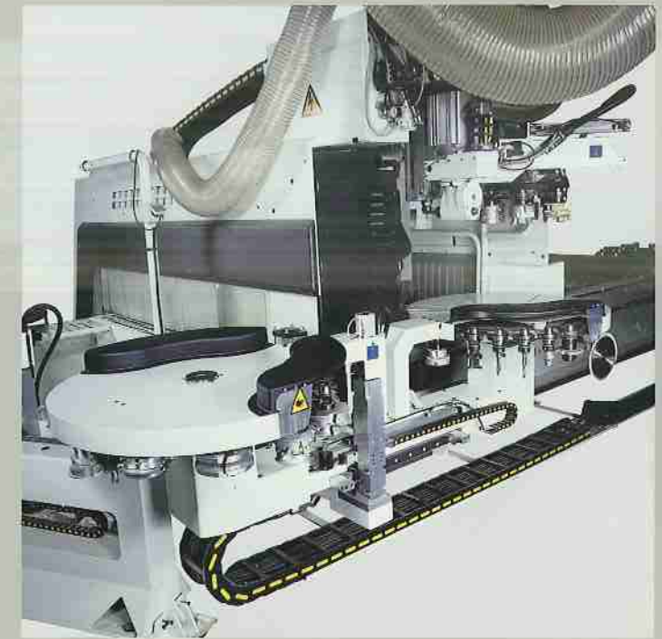
TRM – Additional tool magazine connected to the machine upright. 24 additional tool positions which are changed automatically with those of the Rapid 24.
