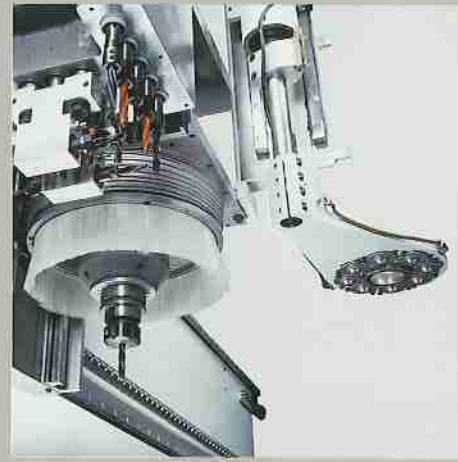
Mechanical presser with ball disc or chrome-plated disc.
