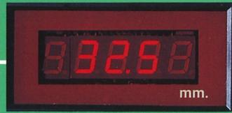
**Digital display of working thickness.**
