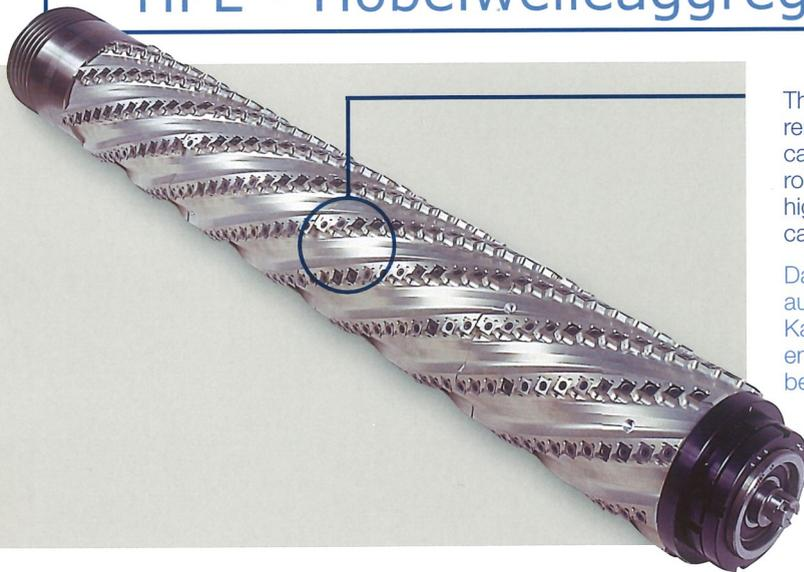
The HPL planer unit is used on solid wood for large-scale chip removal (1 to 3 mm). Under these conditions, without HPL, calibration may be extremely expensive. The number of calibrating rollers and abrasive belts with a grain of 40-60 would actually be high, and the motors power required would also be considerable, causing a great energy consumption.
