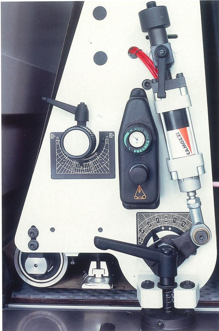
The CS combined unit extends the possibilities for customising the 7S. The roller and the pad on the "CS" can be used separately making this Sandya 7S combined unit highly versatile and suitable for all customer needs.
