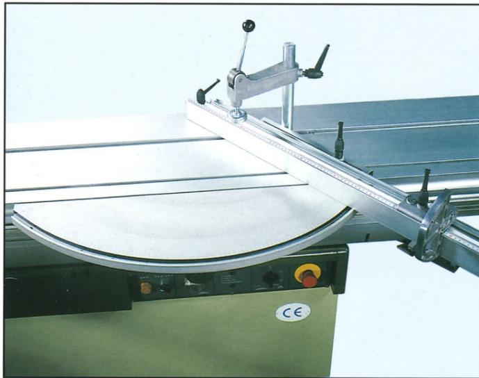
**Mitre unit with compensation for the stop position**
