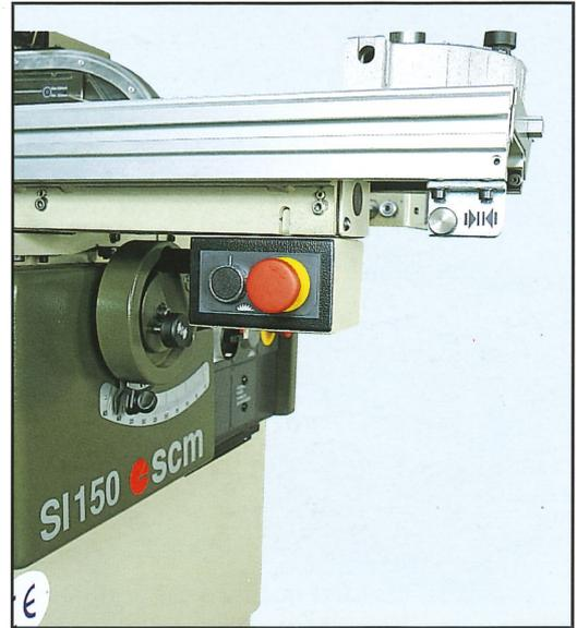
**Front mounted start and stop saw controls**
