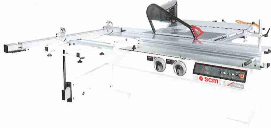
All machines are available in the compact version. The compact version has a 2200 mm sliding carriage, a short frame for squaring cuts and a rip fence capacity of 1000mm.
