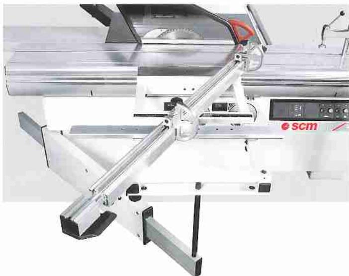
The universal fence permits various operations including as well squaring cuts, rip cuts and mitre cuts on the worktable. The positions of the reference stops are read-off from a metric rule which extends the entire length of the fence.
