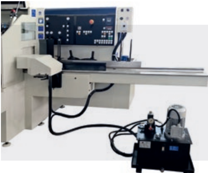
CS1 Hopper feeder provided with a pusher. A serrated roller, driven by an hydraulic device, feeds work pieces continuously.
