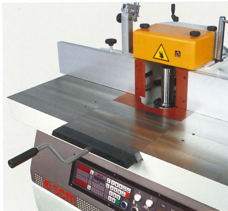
“Fast” sectional worktable The interchangeable worktable sections take the place of traditional table rings and provide maximum workpiece support at all times. The Fast sectional worktable can be adjusted even with the tool already fitted to the machine.
